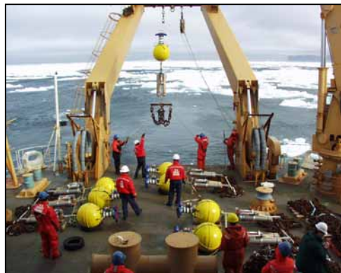
An ADCP being deployed from the aft working deck of the USCGC Healy.
